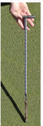
Introducing the new Turf-Tec Tall Tubular Soil Sampler - 1/2 inch diameter sampler (13 mm). This tool that is the thinnest diameter tubular soil sampler in the business. It's entirely made of Stainless Steel. The unit removes a soil sample cores - 6 inches deep at a time. Simply remove from the ground, empty the soil and repeat the sampling process until the 21 inch depth is obtained.
