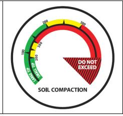
Note: The gauge is engineered to have a positive load, thus the needle does not always contact the pin on the low end of the green scale. This will not affect the readings for either index scale
