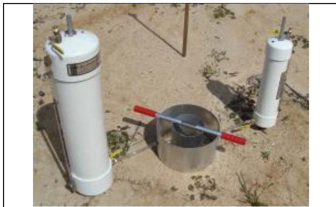
Figure 2A IN12 - Mariotte Tubes are shown - Now both Mariotte tubes are connected to the outside of the unit
