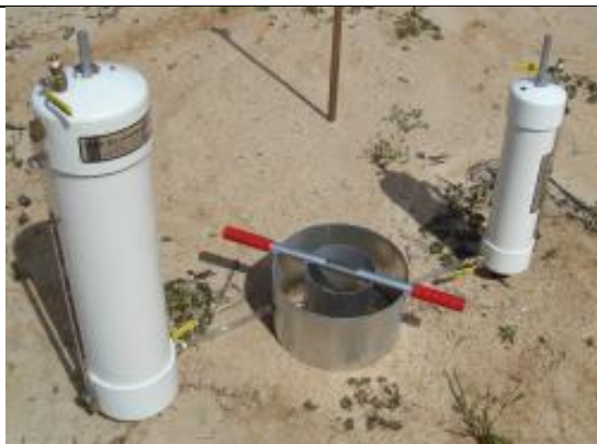
Figure 1 IN8P-W Turf-Tec 6 and 12 inch Infiltration rings and Mariotte Tubes
