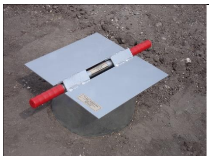
Figure 3 IN11-W Driving Plate shown with IN8P-W Infiltration Rings
