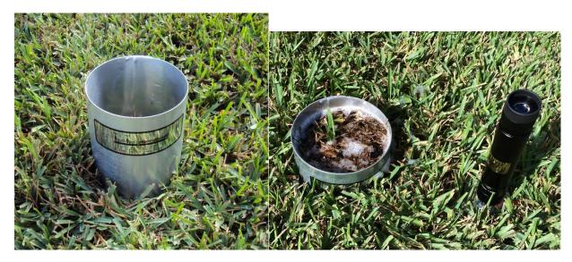
Many insects either float naturally or will float in salty water (e.g., a saturated solution of Epson salts). This tendency can be used to collect and sample insects like chinch bugs in turfgrass. The Turf-Tec Insect Flotation Sampler can be inserted through the thatch in the soil and then filled with water. Within minutes insects will float to the surface where they can be removed or counted to make population level estimates over space and time.
