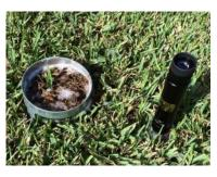
Optional Macroscope 25X shown with the Turf-Tec Insect Flotation Sampler
