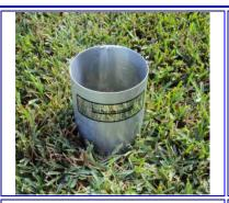
Place the Turf-Tec Insect Flotation Sampler on the area to be tested
