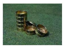
These solid brass sieves are a full eight inches in diameter and are the same type of sieves used by laboratories and Universities for particle size analysis.
