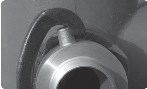
Internal core works on pin-type Hose Couplings or Hydrant Adapters.
