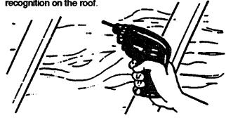
OUTLINING THE HOLE. Draw a circle 14 1/2" in diameter using the guide hole as the center. The carton has a hole template for your convenience.
