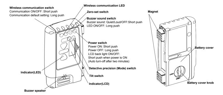
Risk of damage to installation surface of machine, because it uses a strong magnet.
