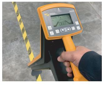
1 The Receiver must be operated facing in the direction of the pipeline or cable.
