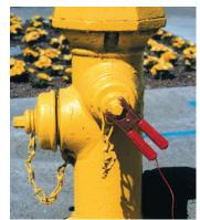
Attach the clamp for the Red cable at a clean spot on conductor.
