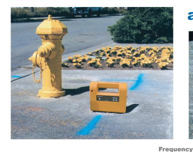
**a** Position the transmitter on the ground over the pipe or cable:
