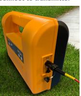
**Connect Red cable to conductor**
