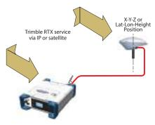
Using a Trimble RTX service in the SP90m requires that you first buy a subscription to this service. On the other hand, the receiver is ready to operate in Trimble RTX mode (dedicated firmware option has been pre-installed at the factory) provided an L-band capable GNSS antenna is used.
