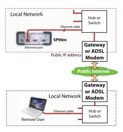
In this configuration, the IT expert should take all the necessary steps for the receiver owner to be able to access the SP90m through the public IP address of the local network. In this case, the IP address shown on the receiver display screen is NOT the one to be used in the web browser.
