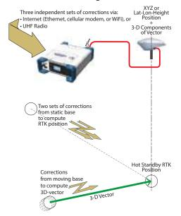
On the receiver's General Status screen, the receiver will display "FIXED" (with short "FLOAT" transition time) when computing a position in Hot Standby RTK mode. The displayed age of corrections is always that of the corrections actually used in the position computation. The computed position is diplayed after pressing .
