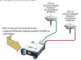
On the receiver's General Status screen, the receiver will display "FIXED" (with short "FLOAT" transition time) when computing a position in RTK DGPS mode for the primary antenna.
