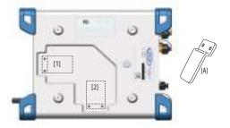
The lug may be secured onto the receiver case in two different ways allowing the receiver to be installed either with its front panel upwards ([1]) or sideways ([2]) (recommended).
