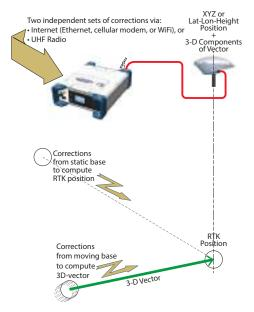
On the receiver's General Status screen, the receiver will display "FIXED" (with short "FLOAT" transition time) when computing a position in RTK mode. The computed RTK position is diplayed after pressing . A new press on this button will display the components of the vector.
