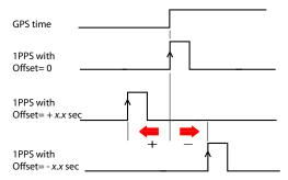
Active edge, i.e. the edge (falling or rising) synchronized with GPS time. (On the diagram above, the rising edge is set to be the active edge)
