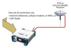
On the receiver's General Status screen, the receiver will display "FIXED" (with short "FLOAT" transition time) or "DGPS" when computing a position respectively in RTK or DGPS mode. The computed position is displayed after pressing ...
