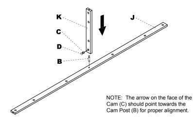
Install the Cam Post (B) into Bottom panel (I). Insert Cams (C) into Koe kick (J) and Bottom slat (K). Attach Bottom panel (I) to Toe Kick (J) and Bottom slat by turning Cams (C).
