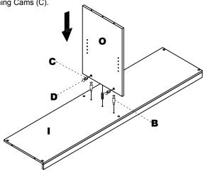
Insert Wood Dowels (A) into Back panel (L). Install the Cam Post (B) into Back panel (L). Insert Cams (C) into center panel (O) and Bottom panel (I). Attach Back panel (L) to center panel (O). Bottom panel (I) and Bottom slat (K) by turning Cams (C).
