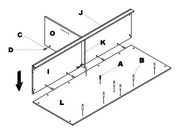
Insert Wood Dowels (A) into Side panel (M & N). Install the Cam Post (B) into Side panel (M & N). Insert Cams (C) into Back panel (L) Bottom panel (I) and Koe kick (J). Attach Side panel (M & N) to Back panel (L). Bottom panel (I) and Koe kick (J) by turning Cams (C).
