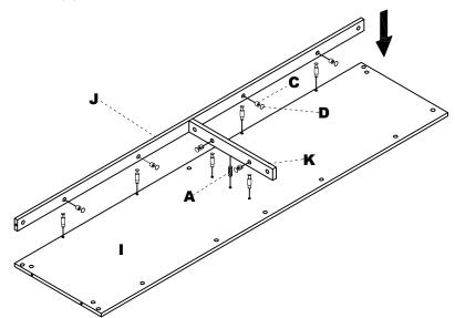
(3) Insert Wood Dowels (A) into center panel (O). Install the Cam Post (B) into Bottom panel (I). Insert Cams (C) into center panel (O) Attach Bottom panel (I) to center panel (O) by turning Cams (C).
