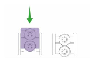
Align your material in the machine, apply downward pressure to the wheel holder and move the cutting head along to create the crease line. Adjust the hand pressure and number of strokes accordingly, you can crease in either direction.
