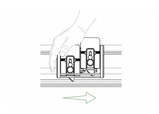
Scoring Acrylic and other plastics can be achieved by setting the blade at minimum depth and running the blade backwards across the surface whilst applying firm downward pressure on the blade holder.
