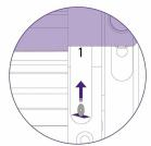
There are four cutting positions on the strip numbered 1 to 4, align the edge of the aluminium end
