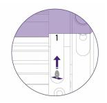
The SmartFold includes an integral polymer cutting strip for use with the Evolution3 Fabric tool head to cut textiles and fragile materials. A simple push button at each end of the bar allows the cutter to be set on any of four cut lines, extending the life of the strip. There is no need for a separate cutting mat.
