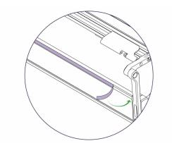
Apply the sightline strip in stages from left to right, ensuring that no wrinkles or bubbles form under the tape.
