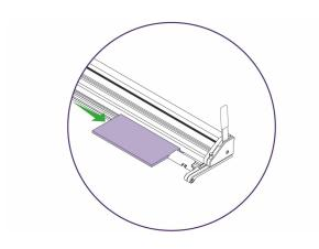
Position the board against the right hand material stop and clamp in place.
