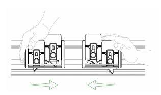
The cutting head can be pulled or pushed to cut the material. Load and align the material to be cut as described in the 'clamping material' section (see how to align and clamp the material >), press down the chosen blade holder whilst pushing/pulling the cutting head along the cutter bar.
