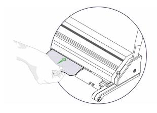
Take a small piece of the material to be cut, clamp it under the cutter bar.
