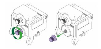
Remove the lower clamping knob.
