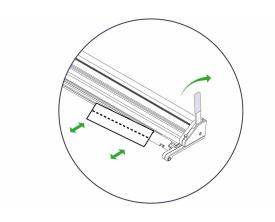
Push the lever to lower the cutter bar so it is only 1-2mm (1/16") above the surface of the material, the closer to the material it is the less lining up error you will get when viewing the cut marks. NOTE: If you find the cutter bar is touching or too low in the middle the cutter bar sag will need adjusting See how to remove cutter bar sag >
