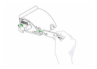
Place the blade cartridge back into the cutting head, press on the end of the blade depth screw to ensure it is located fully in its slot and tighten the blade clamping knob.
