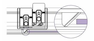
When cutting thick, tough materials such as PVC foam board and fluted plastics such as Correx or Coroplast, set the blade depth so the blade tip protrudes only 1-2mm ( $\frac{1}{16}$ ") through the thickness of the board and cuts from left to right.
