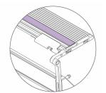
Turn over and re-insert the cutting strip so that the smooth surface is now facing upwards and what was the left hand end goes in first. Push it in nearly all the way, again use a flat edge under the left hand end to raise the strip above the adhesive patch, when in position press the strip onto the patch to prevent it sliding.
