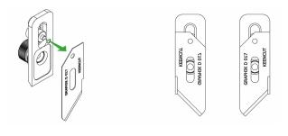
Lift off the blunt blade (if there is one) and replace with a new Graphik blade, check it is facing the correct way for your desired direction of cutting. Place the small pin in the hole at the top of the blade and align with the edge of the clamping plate.
