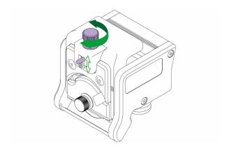
Turn the highlighted screw to adjust the blade pressure (clockwise to reduce). When adjusting you will see the pressure indicator go up and down.
