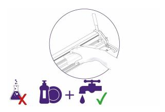
Moisten a cloth with diluted detergent to wipe down the cutter bar and base plate, dry with a cloth.
