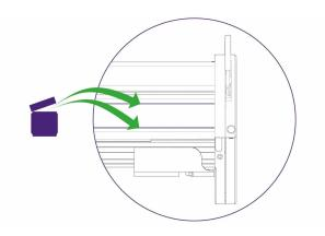
Put a small amount of petroleum jelly (Vaseline) on the scouring surface of a dish washing sponge and rub it up and down the two tracks. Wipe clean any surplus with a dry cloth.
