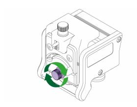
Reassemble with a new blade. Do not over tighten the clamping knob, it is essential that the blade is allowed to rotate whilst cutting.
