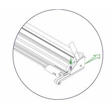
Press and hold down the highlighted button on the right side of the unit. Push the end of the cutter bar away from you.
