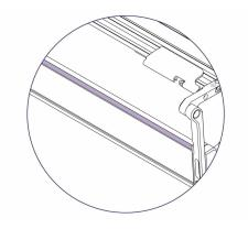
You will see the sightline strip on the underside of the cutter bar.
