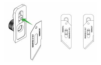
Insert a Graphik blade, check it is facing the correct way for your desired direction of cutting. Place the small pin in the hole at the top of the blade and align with the edge of the clamping plate.
