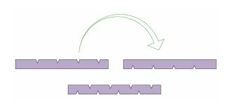
Both sides of the cutting strip can be used, it is important the strip is turned over in the correct orientation. The four tracks are offset to one side so when the strip is turned over correctly the new set of four tracks do not align with the originals.
