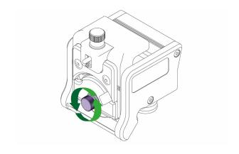
Loosen the clamping knob.
