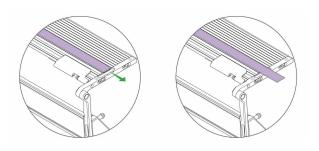
The cutting strip is removed by sliding it to the right, to keep the orientation of the strip correct the left hand end should remain on the left once turned over.
