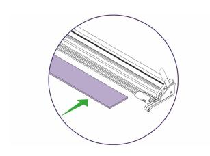
Insert your piece of material and lower the lift and hover so that it is just above the face of the material (as shown previously).
