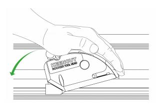
When cutting thicker / more dense materials, ensure the blade depth is adjusted so the blade tip cuts 1-2mm ( $\frac{1}{16}$ ) through the material. Place your hand on the Rocker tool head as shown, press down with your palm to engage the blade.
