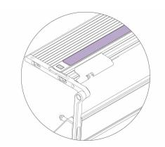
There is a small adhesive patch under the left hand end of the strip to prevent it sliding in use, lift up the strip by sliding a flat edge under the left hand end of the strip and it should then slide to the right. A wide bladed flat screwdriver can be used to help push the strip.
