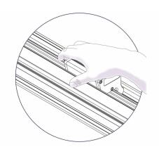
Position the cutting head to start the cut, turn your body to face to the right and place the palm of your right hand on the cutting head.
