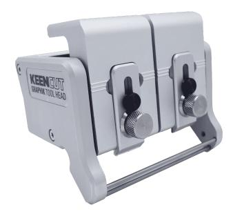
QuikSwap Graphik tool head for Evolution3 cutters, with two individual blade holders for two way cutting. Graphik blades are stronger and more stable than regular blades. Ideal for vinyl, banner, cardboard, PVC foamboard up to 13mm (½"), foamcentred board, corrugated plastic, paper, pop-up and roll-up materials.
