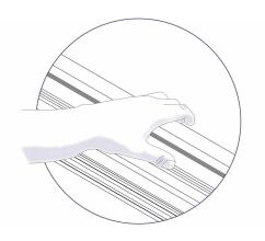
Extra effort can be applied by holding the grip area on the top of the cutter bar with your other hand and using the strength across your shoulders to push. Thicker materials can be cut in several passes.
