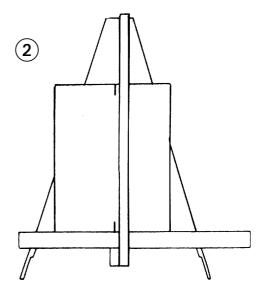
Select the cutting blade on the lower cutting head (see section 6). Cut into the top of the board to produce a cut approximately 3cm (1") long. Disengage the cutter using the cutter release lever. Lower the cutter and make a similar cut at the bottom of the board.
