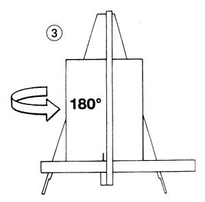
Unclamp and turn the board around (like the page in a book) and place it back in the machine so the same edge is still on the squaring arm but do not clamp it. Align and engage the blade so it enters the previous made cut at the bottom edge of the board. Now apply the clamp.
