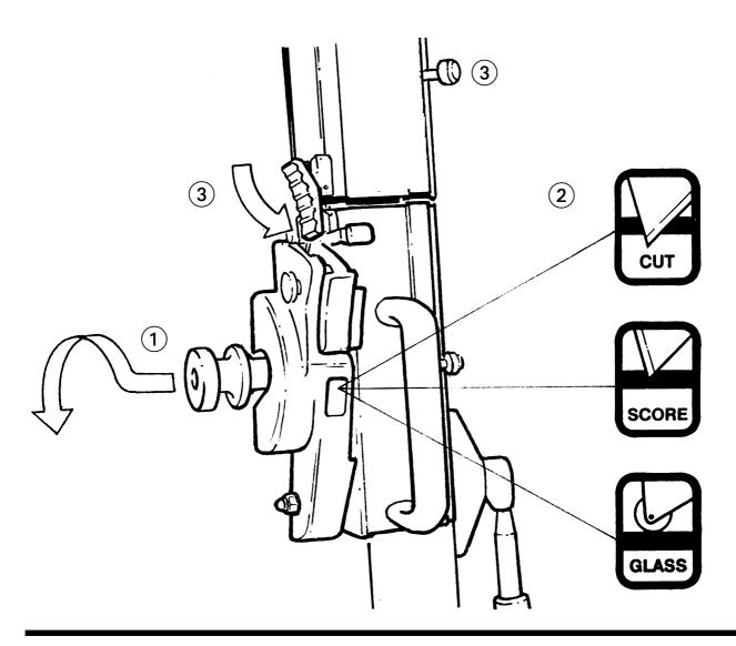
The Excalibur 5000 is fitted with two sliding carriages running on a vertical slideway, each carriage being fitted with a cutting head. The top carriage is fitted with a twin wheel cutter for use with rigid particle boards such as MDF, hardboards and some mount-boards, refer to 'Using the twin wheel cutter' for more details. The lower or Multi-tool cutter head has a rotating turret arrangement where any one of three cutting tools can be selected:
