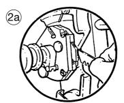
Basic Cutting Technique Select the Cutting Blade position on the turret and clamp the material in the machine.
