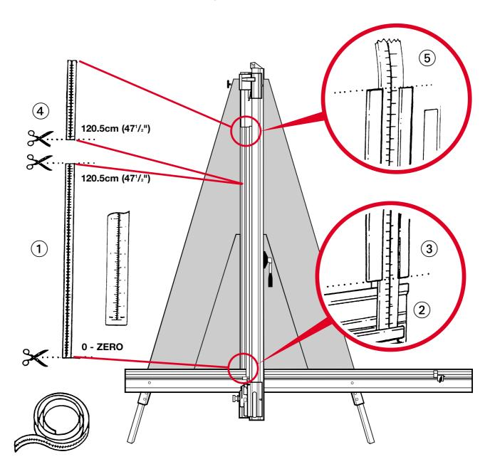
**NOTE:** The *Vertical rules* can be identified from the *Squaring arm rule* by the orientation of the printed measurements – see diagram.
