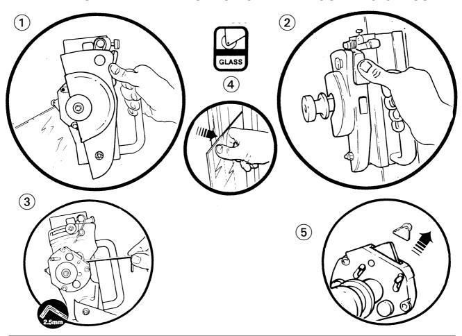
Select the Glass cutter position on the turret, place the glass on the machine loading from the right hand side.
