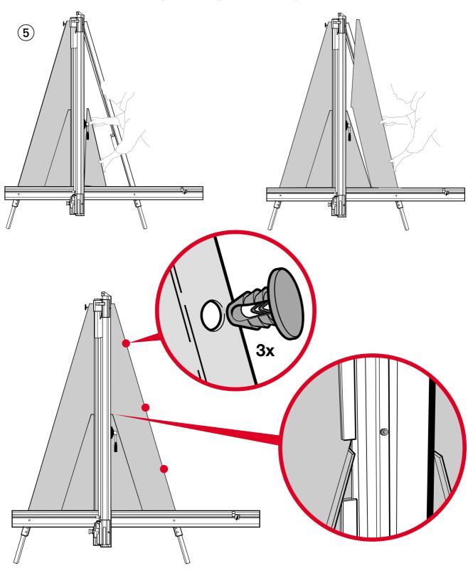
**5.** Repeat for the *Right hand panels*. In place of a vertical groove in the main body the panels have metal strips fixed to the back which grip the edge of the main body as shown.
