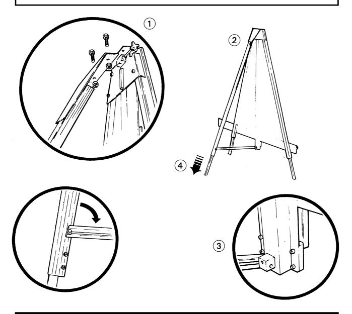
1. Attach the bracket to the top of the machine using the nuts and screws (provided with the main machine).
