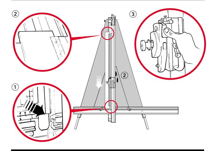
The **Sight-line strip** is fixed to the clamp and then trimmed by the cutting blade to give an accurate guide when cutting to trim lines, the edge of an image or pencil marks. The clamp simply operates by moving the handle in and out, (more information on operating the clamp is given later).
