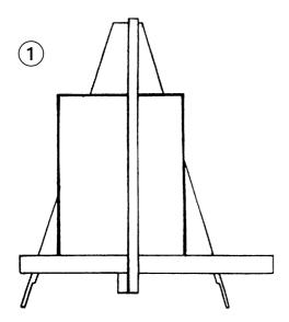
Place the board on the machine vertically as shown and apply the clamp ensuring the bottom edge is in firm contact with the Squaring Arm.
