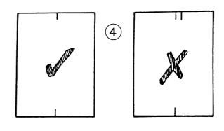
Raise the cutter to the top of the board, if the machine is square the blade should enter the same cut as made previously. If not refer to the following page to make the necessary adjustment.
