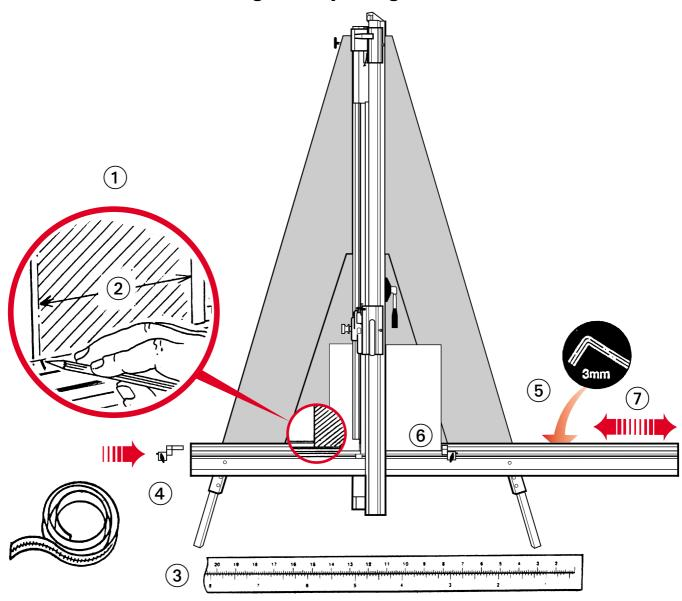
**NOTE:** The Squaring arm rule can be identified from the Vertical rules by the orientation of the printed measurements – see diagram.
