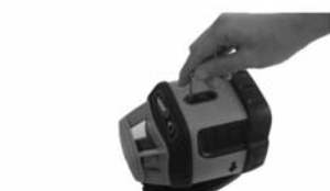
Calibrate the vial using 2.5mm hex wrench
