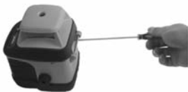
Adjust the fine adjustment bolt
