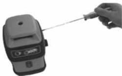
Remove the adjustment-hole bolt
