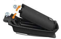
3 Insert four AA batteries, observing polarity.
