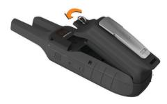
**4** Turn the D-ring clockwise to secure the battery pack onto the device.
