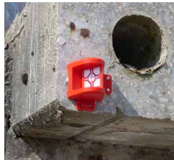
The reflective marker can be perfectly aligned with the measuring instrument at all times.
