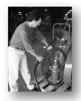
Connect hose coupling to outlet on the extinguisher. Lay hose straight on ground to its full 50-foot. (15.24 m) length. Start first regular loop counter-clockwise by placing between side brackets and over the top bracket.
